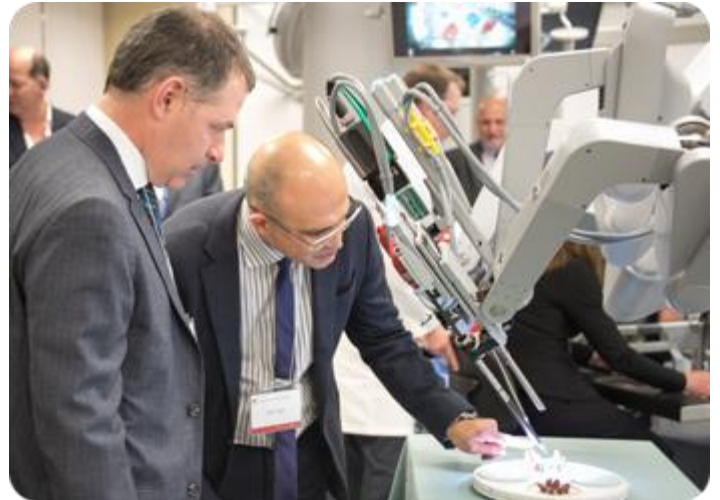
Photo: LHSC Chair/Chief of Cardiac Surgery Dr. Bob Kiaii (right) explains to donor Jamie Crich how a two-camera setup in one of the da Vinci's four robotic arms produces high-resolution 3D images to help guide surgeons.
